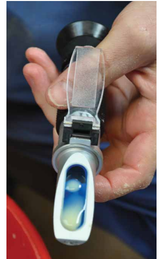
Figure 2: Brix refractometer needs only a drop of colostrum to assess quality.
